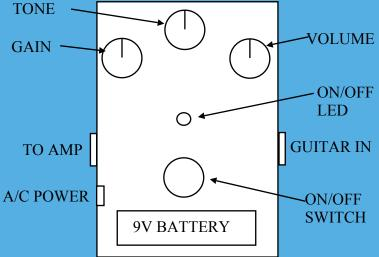
GAIN: CONTROLS A WIDE GAIN RANGE VOLUME: CONTROLS THE VOLUME MIX CRASH: ADJUSTS THE TONE FROM BASS (LEFT) TO TREBLE (RIGHT) A/C POWER JACK REQUIRES 9V, 2.1mm, NEGATIVE CENTER POWER SUPPLY REMOVE BACK PLATE TO ACCESS 9V BATTERY CLIP
