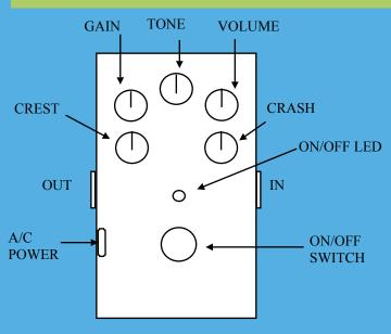
GAIN: Controls a wide gain range TONE: Controls the tone sweep VOLUME: Controls volume range
