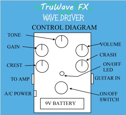
GAIN: CONTROLS A WIDE GAIN RANGE VOLUME: CONTROLS THE VOLUME MIX
